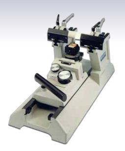
**INCLUDES**: 0-40µm feed screw with 1µm increments; Manual gross advance/rewind facility; angled, tilted knife holder with indicator scale; full width integral knife guards; Automatic retraction of approx. 50µm on return stroke; standard vice or quick release cassette holder; Fixed adaptor; Knife cleaning brush, (4) Allen keys, microtome oil and operating manual
